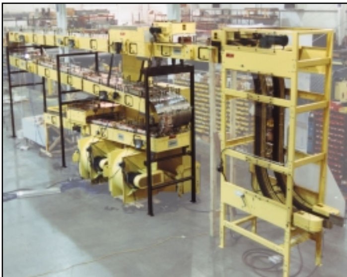
AIR DECK™ Conveyor in “Z” Decline Configuration
